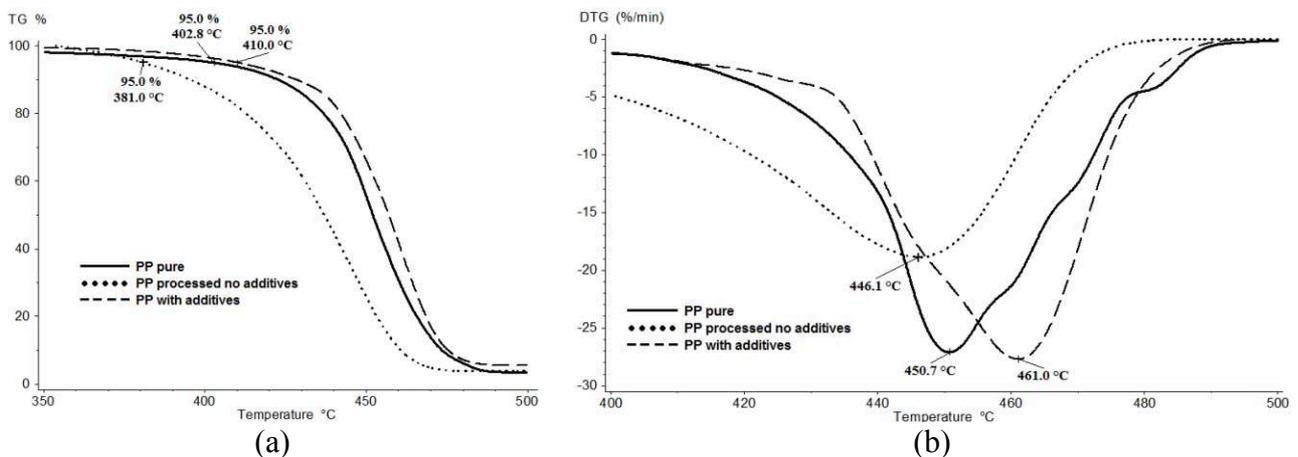
Fig. 3 – (a) Curve of mass loss versus temperature of pure PP, PP processed no additives and PP with additives. (b) Curve of the first derivate of pure PP, PP processed no additives and PP with additives and illustration of the maximum degradation temperature.
