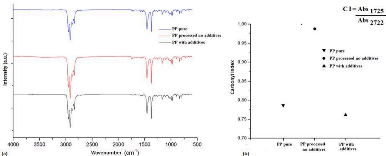
Fig. 2 – FTIR spectra for the surfaces of (a) pure polypropylene, (b) processed polypropylene and (c) polypropylene with additives.
