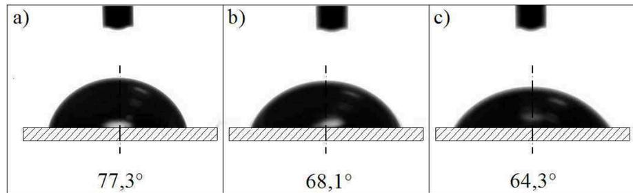
Fig. 1 – The contact angle for the surfaces of (a) pure polypropylene, (b) processed polypropylene and (c) polypropylene with additives.
