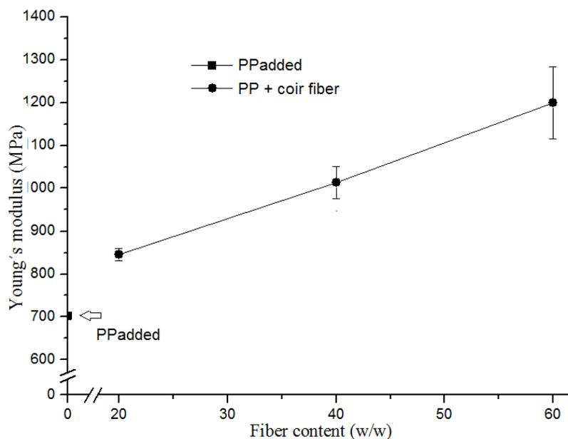
Fig. 4 – Young's modulus for polypropylene containing additive and polypropylene composites according to fiber types and filler. The points are the mean  $\pm$  standard deviations (SD) of ten determinations.
