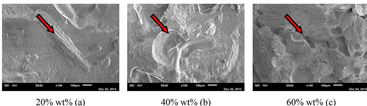
Fig. 5 - Images photomicrographs of PP composites with coir (100x).
