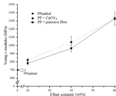
Fig. 2 – Young's modulus for PP containing additive and PP composites according to piassava fiber and CaCO<sub>3</sub> filler. The points are the mean  $\pm$ SD of ten determinations.
