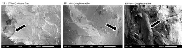
Fig. 4 - Photomicrographs of PP composites with 20, 40, 60 wt% piassava fibers.
