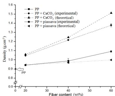
Fig. 1 – Determination of theoretical and experimental data density for PP and PP composites according to piassava fiber and CaCO<sub>3</sub> filler. The points are the mean  $\pm$ SD of five determinations.
