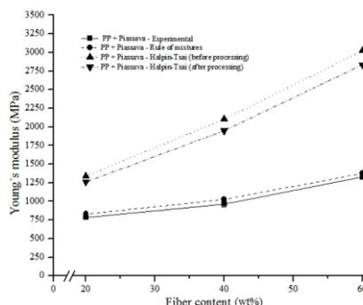
Fig. 3 – Determination of modulus for rule of mixtures and Halpin-Tsai equations for composites with piassava fiber.
